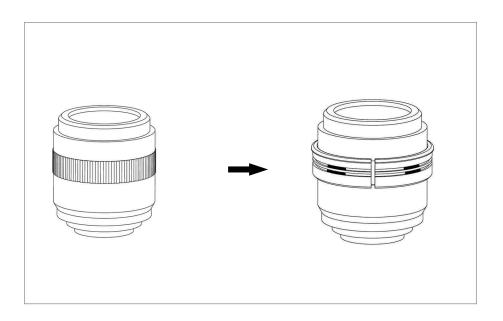
Keep the lens rubber ring on while installing the plastic c-ring onto the zoom ring area.
