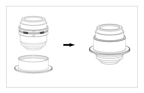
2. Insert the gear ring of C60-f on the plastic c-ring, as shown in the diagram, until it reachs the flange of the plastic c-ring.
