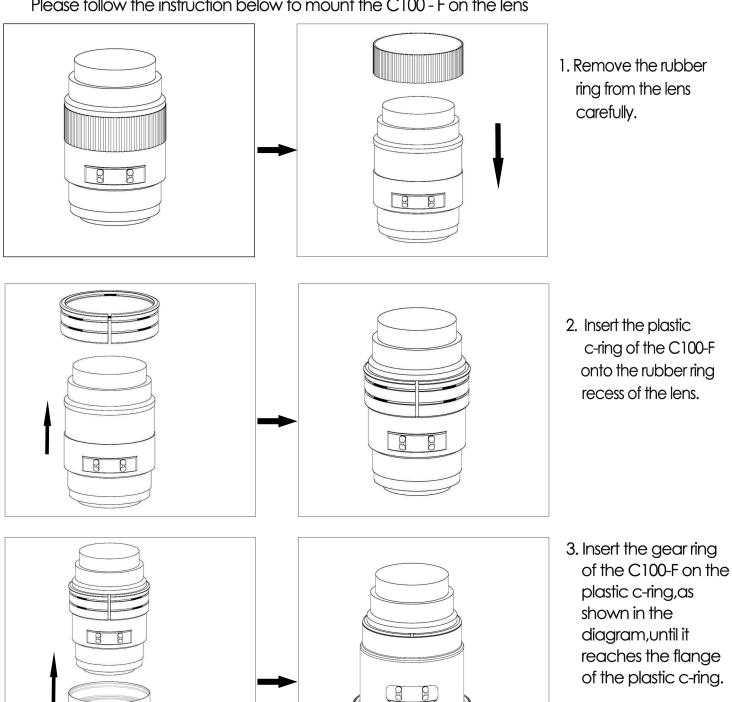
4. The tightness between the C100-F gear and the lens can be adjusted by removing or adding rubber grips on either sides of the plastic c-ring, spare rubber grips are included in the package.
