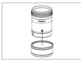
2. Insert the plastic c-ring as shown and place it onto the rubber ring recess of the lens.
