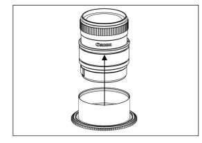
3. Insert the gear of C18135IS-Z on the plastic c-ring until it reaches the flange of the plastic c-ring.
