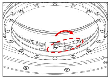
Turn the locking device sideways into the recess. Ensure that the locking device is secured inside the recess and the extension ring is securely locked with the port.
