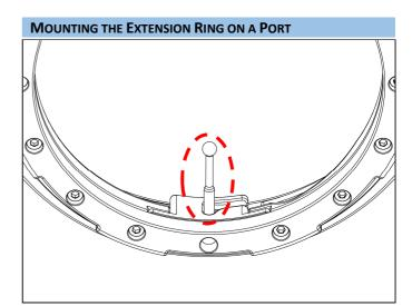
Confirm that the extension ring is unlocked, with the locking pin pointing upwards as shown.
