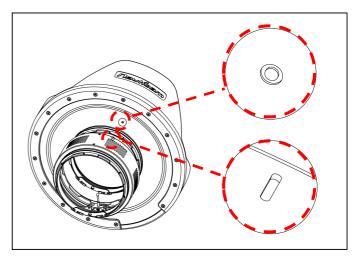
Align the "I" mark on the extension ring with the WHITE dot on the port.
