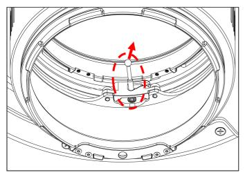
To lock the extension ring, push the locking pin inwards.
