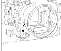
4. Turn the port locking lever to the outward position.
