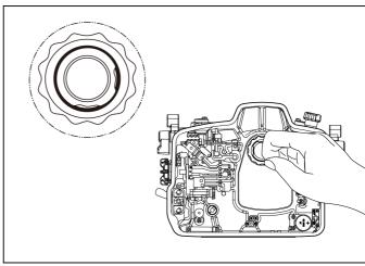
Remove the retainer O-ring of the viewfinder inside the rear half of the housing by making use of the recess on the viewfinder.
