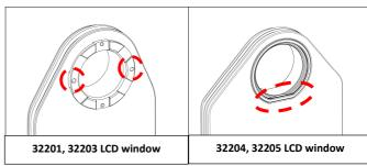
Align the viewfinder's alignment pins/ slot with the holes/ slot of the sleeve in the LCD display window.
