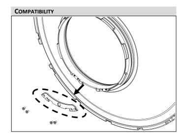
This port is backwards compatible with other N120 extension rings. A user installable locking tab is pre-installed for this purpose.
