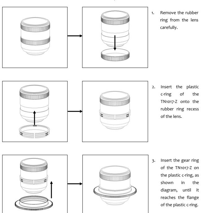
4. The tightness between the TN1017-Z and the lens can be adjusted by removing or adding rubber grips on either sides of the plastic c-ring. Spare rubber grips are included in the package.
