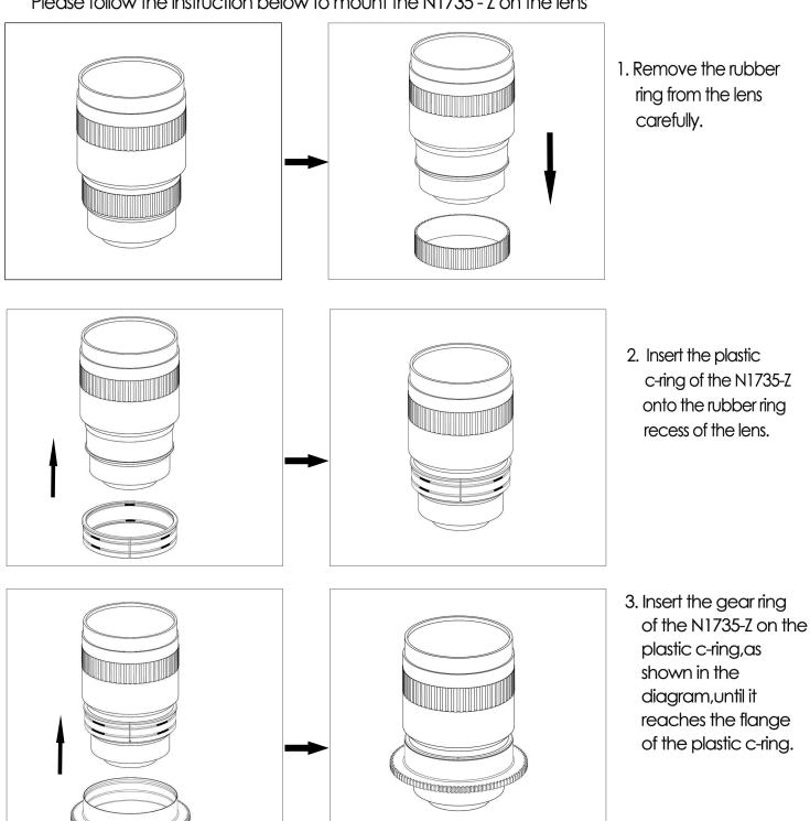
4. The tightness between the N1735–Z gear and the lens can be adjusted by removing or adding rubber grips on either sides of the plastic c-ring, spare rubber grips are included in the package.
