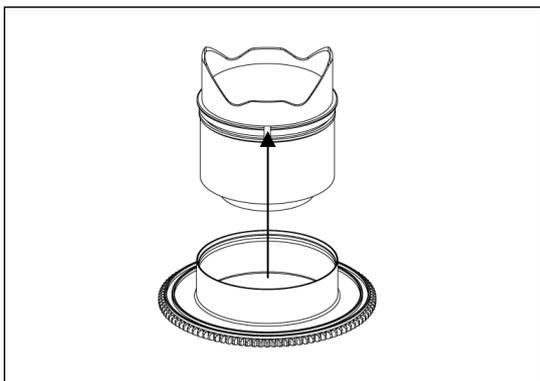
3. Insert the gear of N10.5-F on the plastic c-ring until it reaches the flange of the plastic c-ring.
