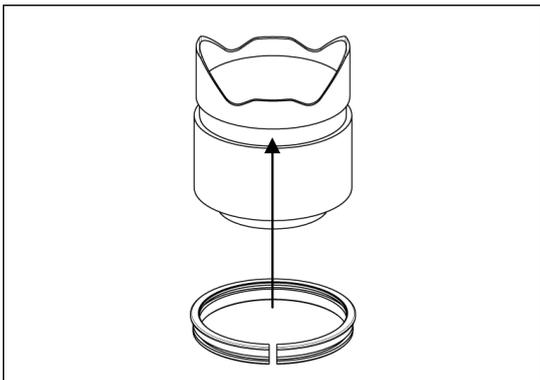
2. Insert the plastic c-ring as shown and place it onto the rubber ring recess of the lens.
