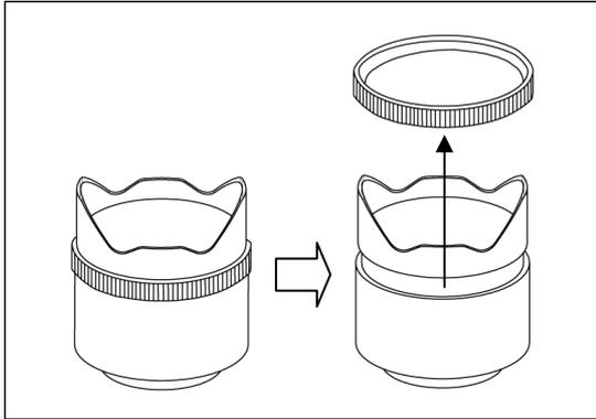
1. Remove the rubber ring from the lens carefully.
