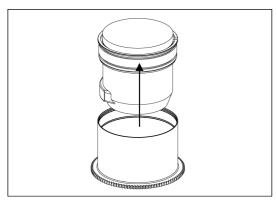
2. Insert the gear of N2485-Z on the plastic c-ring until it reaches the flange of the plastic c-ring.
