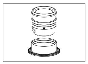
2. Insert the gear of SN1770OSC-Z on the plastic c-ring until it reaches the flange of the plastic c-ring.
