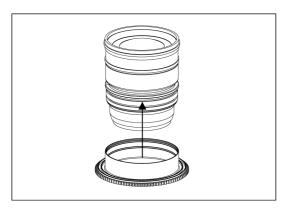
Insert the gear of N1835-Z on the plastic c-ring until it reaches the flange of the plastic c-ring.
