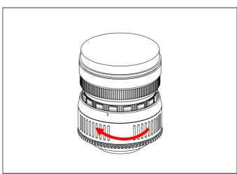
Tighten the zoom/focus gear by turning the locking ring clockwise while holding the toothed part firmly, until it cannot go in any further.
