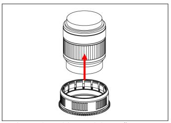
Insert the gear as shown and place it over the lens zoom/focus ring.
