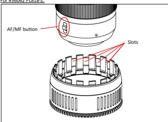
Align the AF/MF button on the lens with one of the slot on the zoom gear. Insert the gear as shown all the way up until it stop.
