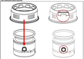
Align the "opening" of the gear with the button on the lens barrel. Insert the gear of N6.713-Z as shown and place it over the lens zoom ring.
