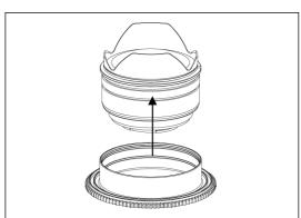
2. Insert the gear of SN15-F on the plastic c-ring until it reaches the flange of the plastic c-ring.
