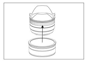
1. Insert the plastic c-ring as shown and place it over the lens rubber focus ring.
