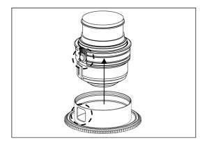
2. Align the "opening" of the gear with the button on the lens barrel. Insert the gear of N1855VRII-Z on the plastic c-ring until it reaches the flange of the plastic c-ring.
