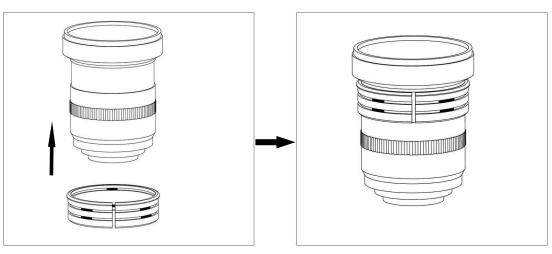
2. Insert the plastic c-ring of the C1022-Z onto the rubber ring recess of the lens.
