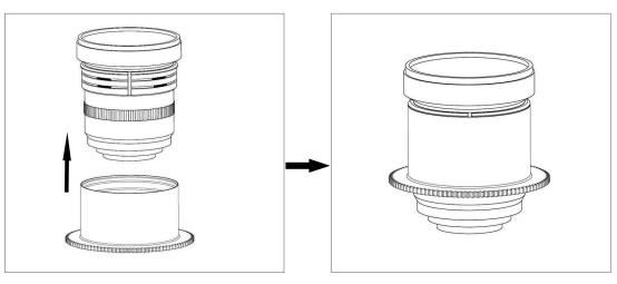
3. Insert the gear ring of the C1022-Z on the plastic c-ring, as shown in the diagram, until it reaches the flange of the plastic c-ring.
