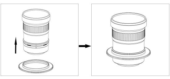
3. Insert the gear ring of the C1740-Z on the plastic c-ring, as shown in the diagram, until it reaches the flange of the plastic c-ring.
