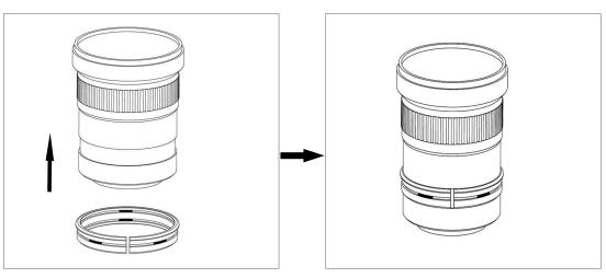
2. Insert the plastic c-ring of the C1740-Z onto the rubber ring recess of the lens.
