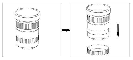
Remove the rubber ring from the lens carefully.
