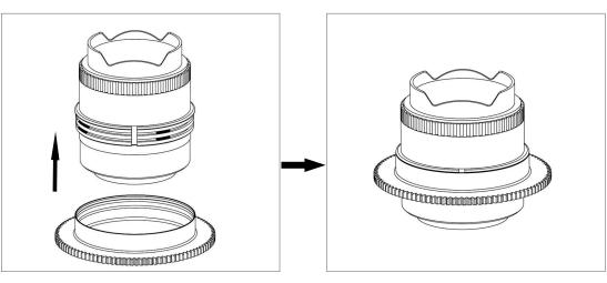
3. Insert the gear ring of the TC1116-Z on the plastic c-ring, as shown in the diagram, until it reaches the flange of the plastic c-ring.
