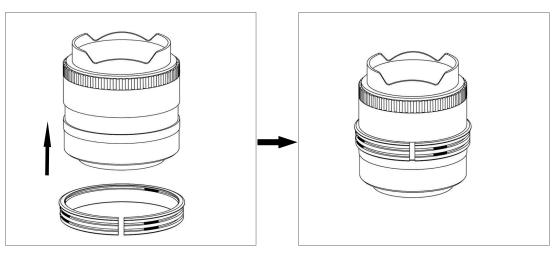
2. Insert the plastic c-ring of the TC1116-Z onto the rubber ring recess of the lens.
