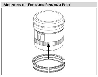
Insert the plastic c-ring as shown and place it over the lens rubber zoom ring.
