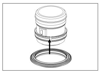
Insert the gear of C815-Z on the plastic c-ring until it reaches the flange of the plastic c-ring.
