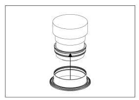
2. Insert the gear of C815-Z+1.4 on the plastic c-ring until it reaches the flange of the plastic c-ring.
