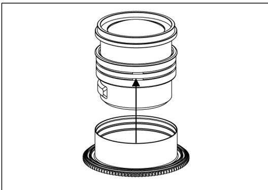
2. Insert the gear of SC1770OSC-Z on the plastic c-ring until it reaches the flange of the plastic c-ring.
