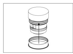
2. Insert the gear of C815-F on the plastic c-ring until it reaches the flange of the plastic c-ring.
