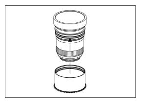
3. Insert the gear of C1635II-F on the plastic c-ring until it reaches the flange of the plastic c-ring.
