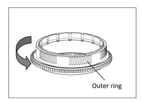
Loosen the zoom gear by turning the outer ring anticlockwise while holding the toothed part firmly, until it can be inserted onto the lens.
