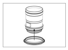
2. Insert the gear of C2470f4-Z on the plastic c-ring until it reaches the flange of the plastic c-ring.
