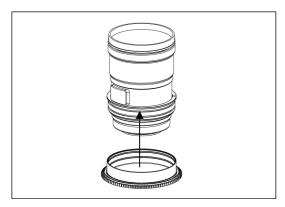
2. Insert the gear of C24105-Z on the plastic c-ring until it reaches the flange of the plastic c-ring.
