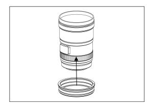
1. Insert the plastic c-ring as shown and place it over the lens rubber zoom ring.
