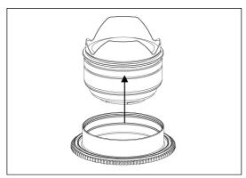
2. Insert the gear of SC15-F on the plastic c-ring until it reaches the flange of the plastic c-ring.
