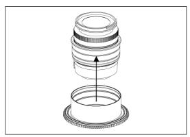
2. Insert the gear of C1855ISSTM-Z on the plastic cring until it reaches the flange of the plastic cring.
