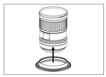
Insert the gear of C1635f4-Z on the plastic c-ring until it reaches the flange of the plastic c-ring.
