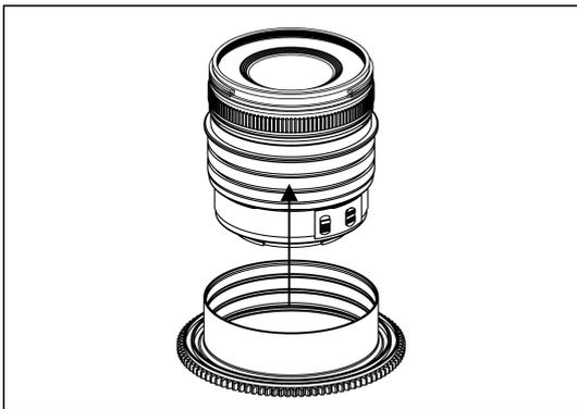
2. Insert the gear of C1018-Z on the plastic c-ring until it reaches the flange of the plastic c-ring.
