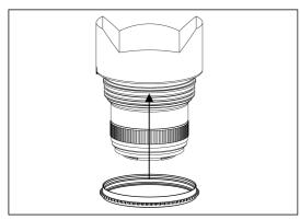
2. Insert the gear of C1124-F on the plastic c-ring until it reaches the flange of the plastic c-ring.
