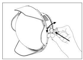
2. Engage the gear by pushing the knob inwards, then turn the knob both ways to check if the lens focuses.
