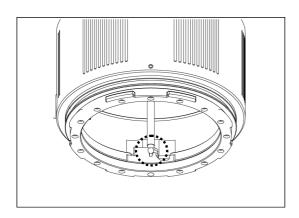
Confirm that the extension ring is unlocked, with the locking device pointing upwards as shown.
