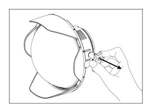
Make sure the control knob is at its most outwards position before mounting/ un-mounting the port. The knob should be left at this position until it is made sure that the lens and focus gear is properly installed.
