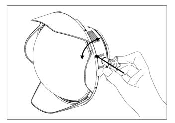
2. Engage the gear by pushing in the knob, then turn the knob both ways to check if the lens focuses.
