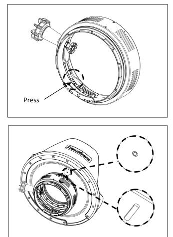
Confirm that the extension ring is unlocked, Press the RED bar to unlock the locking device of the extension ring.
