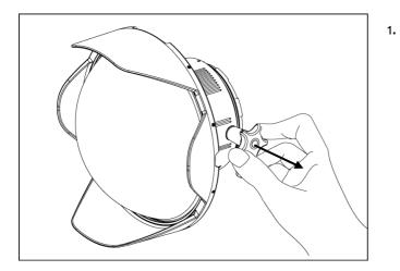
Make sure the control knob is at its most outwards position before mounting/ un-mounting the port. The knob should be left at this position until it is made sure that the lens and focus gear is properly installed.
