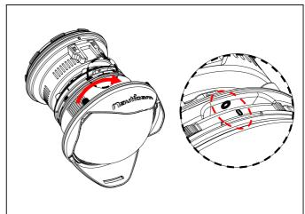
Turn the lens clockwise until the "I" mark on the lens aligns with the WHITE dot on the converter and a "click" sound is heard.
