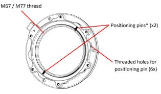
\*There are two alignment pins at the bottom of the holder, by relocating the two screws to the threaded holes around the holder, the position of the holder can be changed.
