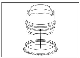
2. Insert the gear of P8-F on the plastic c-ring until it reaches the flange of the plastic c-ring.
