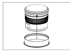
2. Insert the gear of P1235-F on the plastic c-ring until it reaches the flange of the plastic c-ring.
