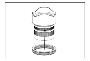
1. Insert the plastic c-ring as shown and place it over the lens focus ring.
