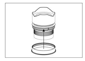
2. Insert the gear of P714-F on the plastic c-ring until it reaches the flange of the plastic c-ring.
