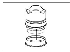
2. Insert the gear of P714-Z on the plastic c-ring until it reaches the flange of the plastic c-ring.
