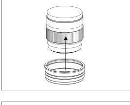
1. Insert the plastic c-ring as shown and place it over the lens zoom ring.
