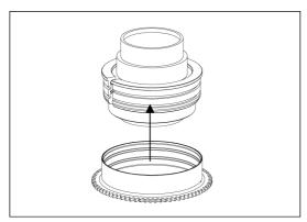
2. Insert the gear of P1232-Z on the plastic c-ring until it reaches the flange of the plastic c-ring.
