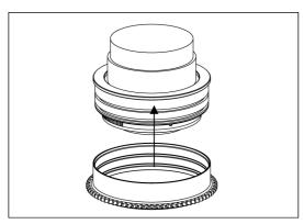
2. Insert the gear of O1442EZ-Z on the plastic c-ring until it reaches the flange of the plastic c-ring.
