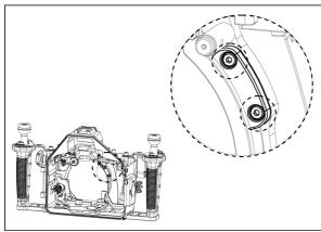
Locate the port stopper block in the front housing. Remove the plastic block by unscrewing the two screws. Replace the plastic block with the supplied metal block then fastened by tightening the two screws.
