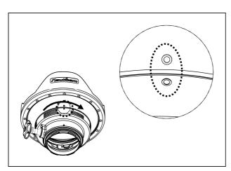
3. Turn the extension ring clockwise until the white dot on the extension ring aligns with the white dot on the port.
