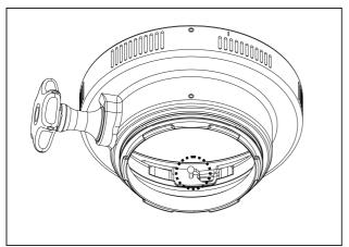
Confirm that the extension ring is unlocked, with the locking device pointing upwards as shown.
