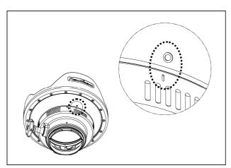
2. Align the "I" mark on the extension ring with the WHITE dot on the port. Then gently push the extension ring towards the port until it cannot go in any further
