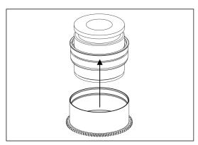
2. Insert the gear of P1445-Z on the plastic c-ring until it reaches the flange of the plastic c-ring.
