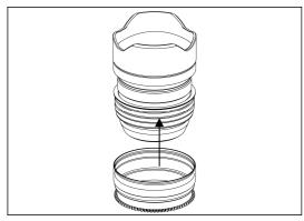
2. Insert the gear of O714-Z on the plastic c-ring until it reaches the flange of the plastic c-ring.
