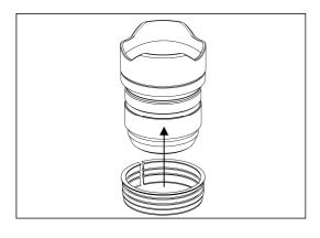
1. Insert the plastic c-ring as shown and place it over the lens zoom ring.
