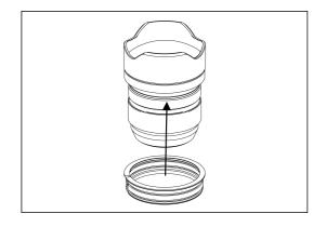
1. Insert the plastic c-ring as shown and place it over the lens focus ring.
