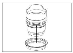
2. Insert the gear of O714-F on the plastic c-ring until it reaches the flange of the plastic c-ring.
