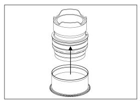
2. Insert the gear of O8-F on the plastic c-ring until it reaches the flange of the plastic c-ring.
