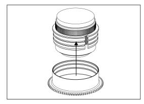
2. Insert the gear of P1442II-Z on the plastic c-ring until it reaches the flange of the plastic c-ring.
