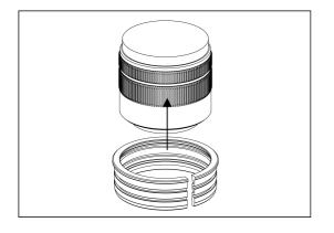
1. Insert the plastic c-ring as shown and place it over the lens zoom ring.
